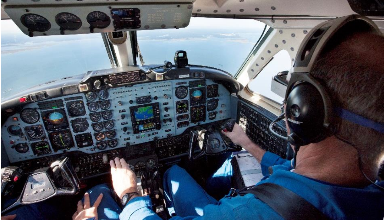
Figure 4: BE-200 Cockpit with Evaluation Pilot in Right Seat wearing the HWD
