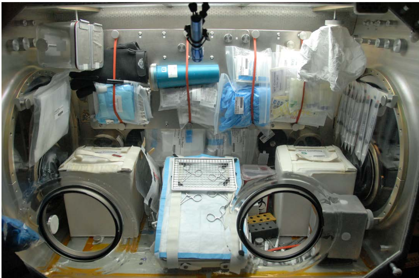
MSG (Ground Unit) with Rodent Research Hardware Setup (single crew ops)
