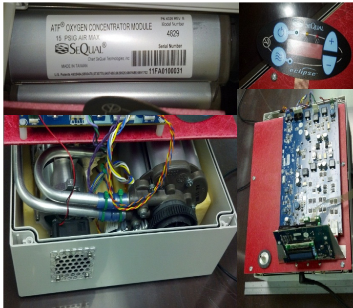
Figure 4.—Top left image shows packed bed module from SeQual, and bottom left image shows same packed bed (right) next to the compressor (left). Both sit on a bed of foam to provide vibration and noise dampening. Shown on the lower right is the exposed top circuitry and a display of the flow rate. The image on the top right shows the touchpad control on the prototype that toggled between off, 6, 3, 2, and 1 lpm.
