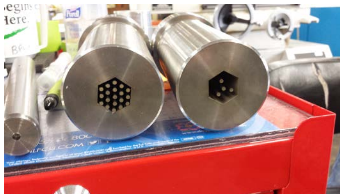
Above: 19 and 4-hole NERVA fuel element extrusion dies; Left: Graphite extruder with vent lines installed for DU capability
