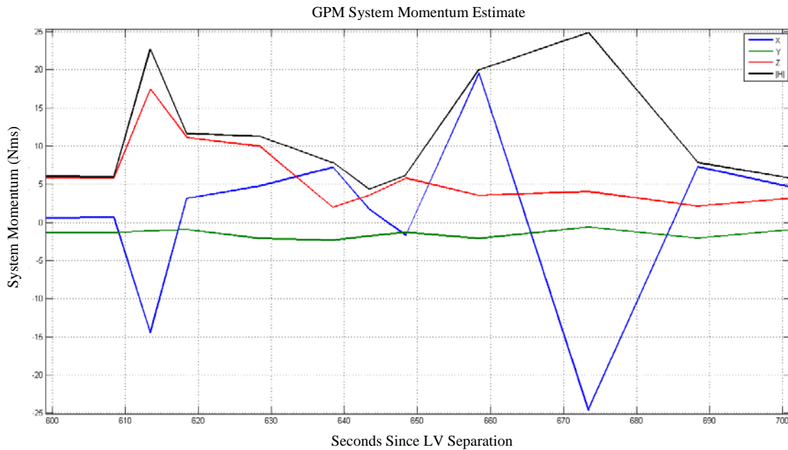
Figure 2: System Momentum Estimate During Solar Array Deployment.
