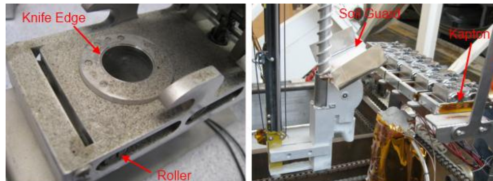
Figure 7: At left, the sample collection mechanism after Test 1. Soil falling from the upper portion of the auger contaminated the knife edge seal. At right, the mitigation techniques used in Test 2 including the soil guard and kapton tape over the rollers.
