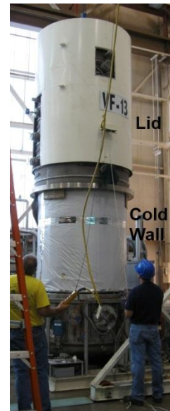
Figure 1: The VF13 chamber with the lid being lowered over the cold wall.
