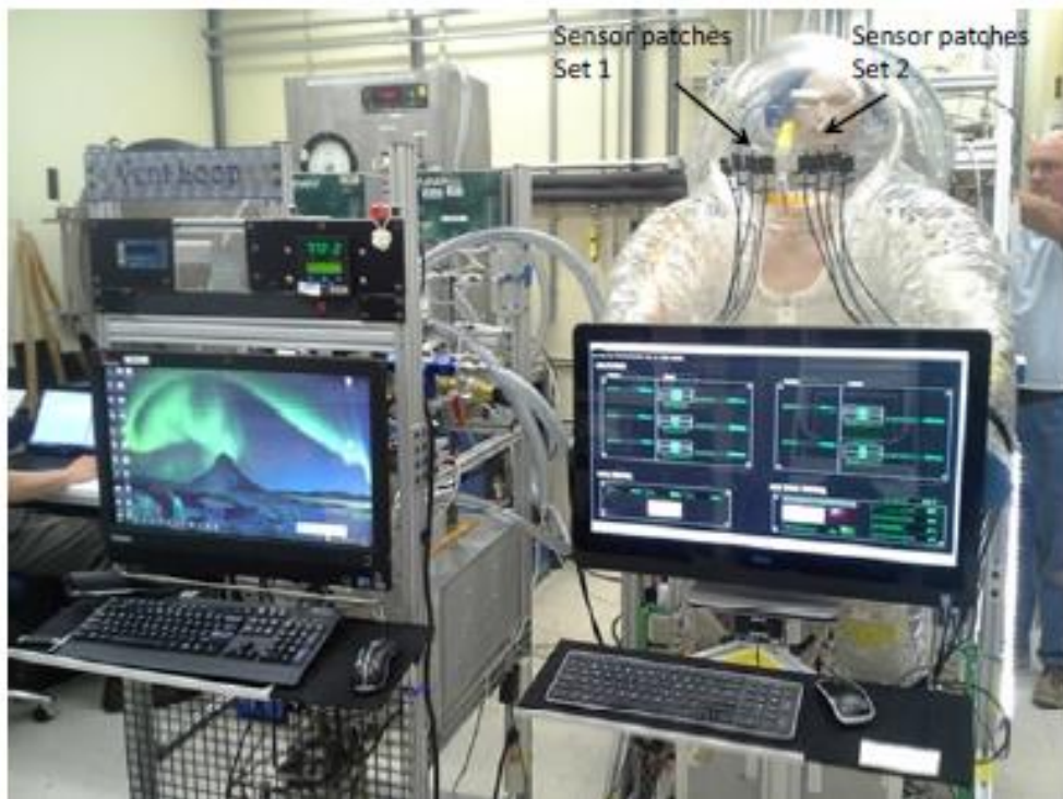
Figure 9. Vent Loop (left) and SMTA (right) Setup for Patch Sensor Testing
