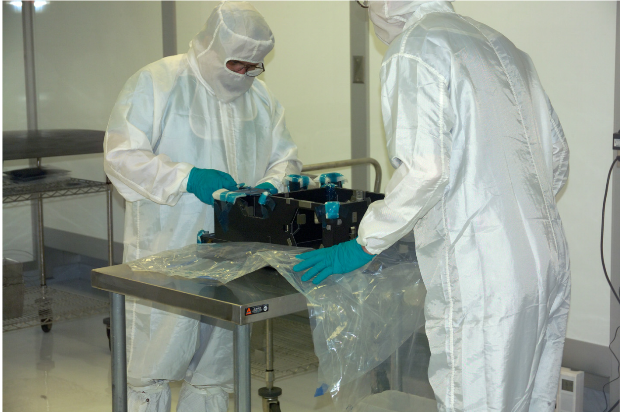
Figure 16 PPE used for Handling Composite Structure in a Clean Room
