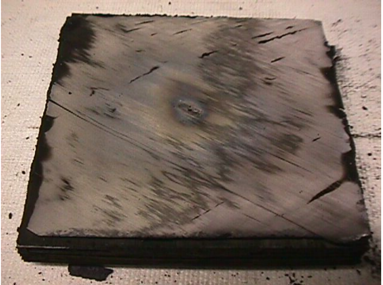
Figure 14 Forensics on Post-Fire Coupon
