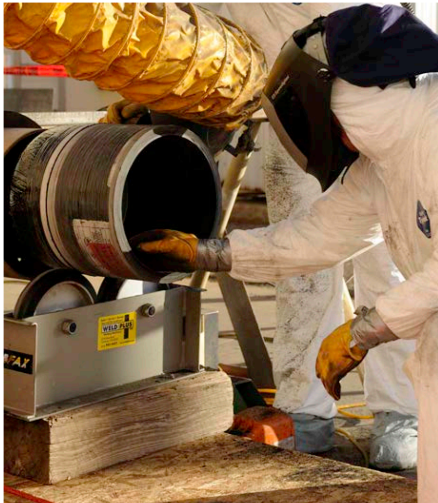
Figure 15 Proper Methods to Prevent Exposure at Cuffs and Ankles
