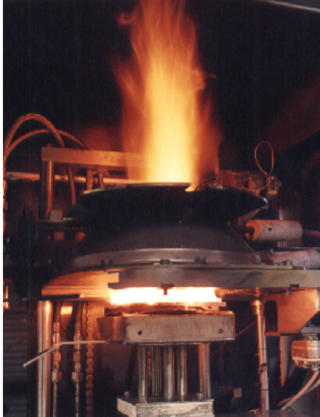
Figure 12 Combustion of Composite Sample for Thermal De-Ply Analysis
