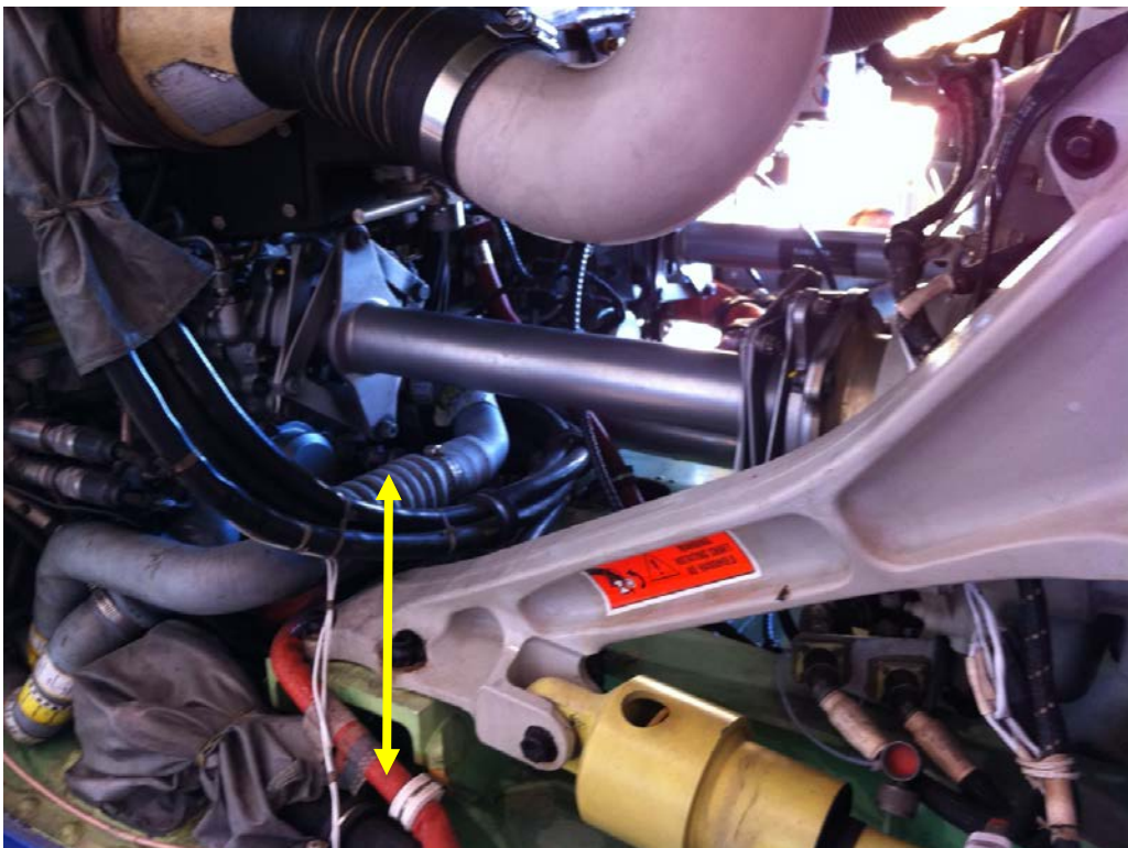
Figure 27. Typical rotorcraft installation. Roof panel is in green below the strut. Yellow arrow denotes oscillatory transverse force.
