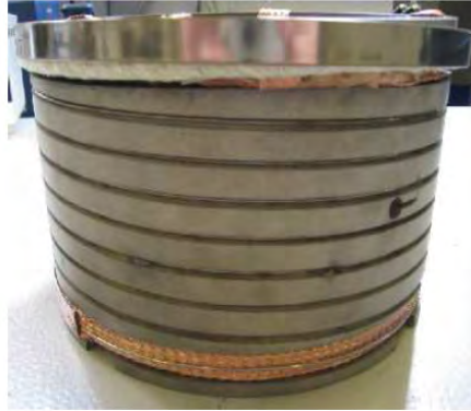
Figure 124.—University of Manchester SFCL Windings on Slotted Former (Ref. 168).
