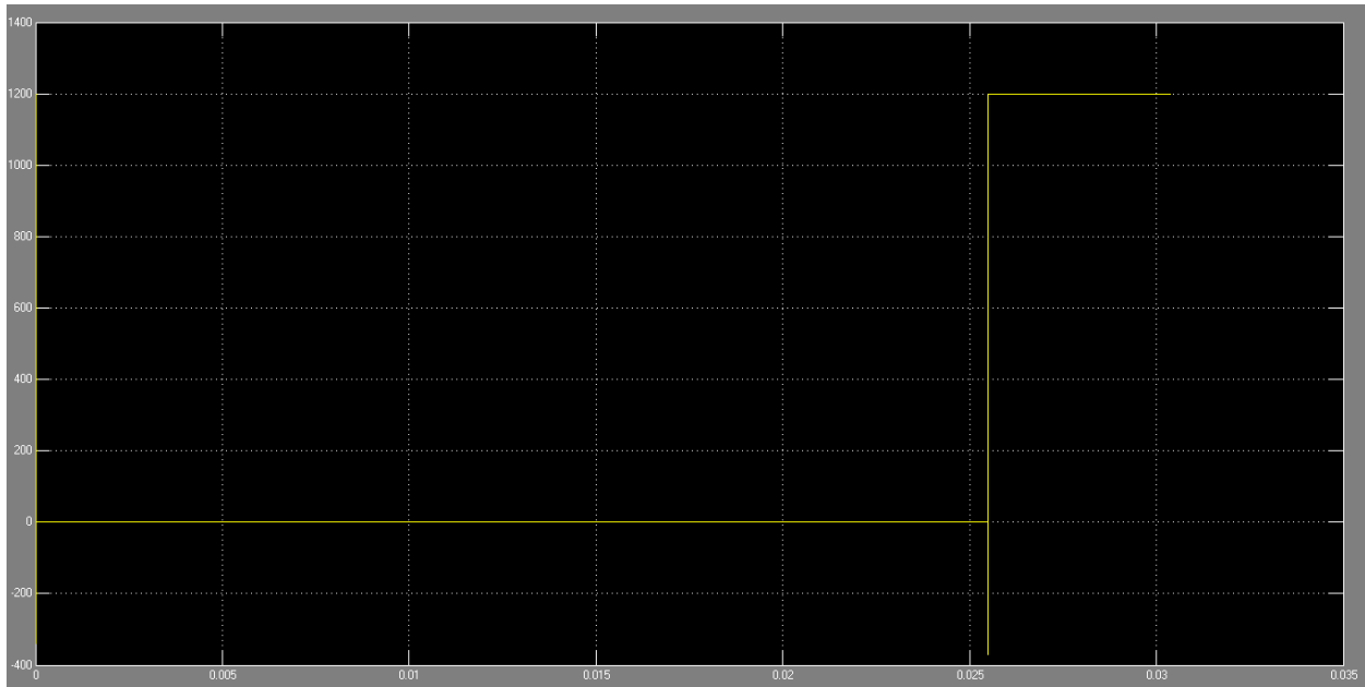
Figure 225.—Right Engine Failure SMES Discharge.
