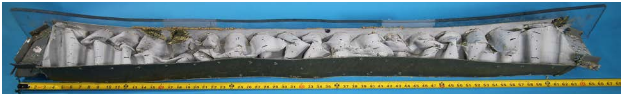
Figure 23. Photograph of the conusoid energy absorber, removed from the test article. Note that the conusoid is lying on its side with a portion of the polycarbonate floor still attached.
