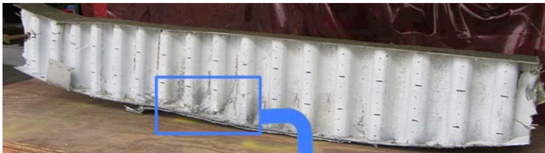
(a) Post-test photograph of the conusoid energy absorber, rear view looking forward.
