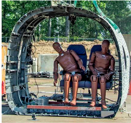
(a) Post-test photograph of the barrel section.
