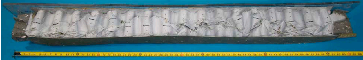
Figure 27. Photograph of the sinusoid foam sandwich energy absorber, removed from the test article. Note that the subfloor section is lying on its side with a portion of the polycarbonate floor still attached.
