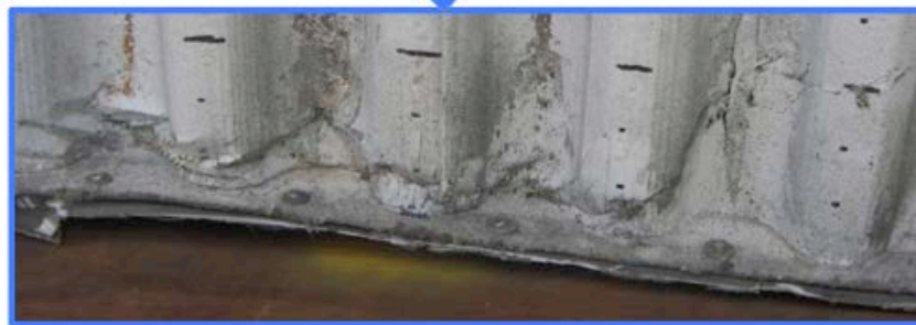
(b) Sinusoid energy absorber, rear view looking forward. Inset shows regions of crush initiation.
