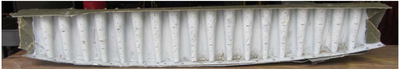
(a) Post-test photograph of the conusoid energy absorber, rear view looking forward.
