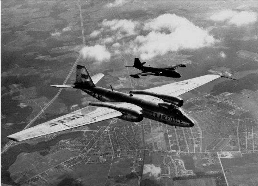
The Martin RB-57D was based on the B-57 light, twin-engine bomber, but with improved engines and a longer wingspan. (U.S. Air Force)
