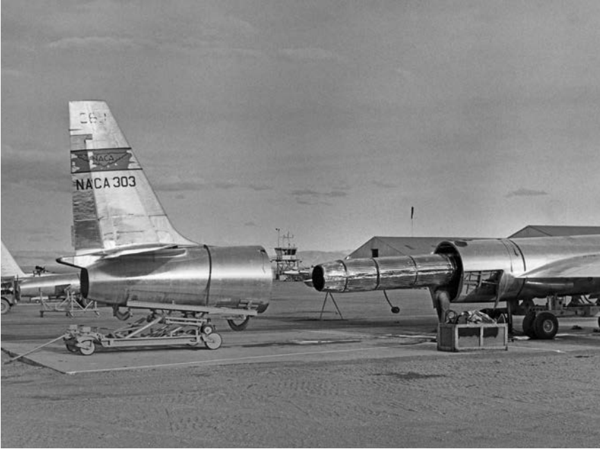
The tail-fuselage interface was designed for ease of assembly and maintenance. (Laughlin Heritage Foundation)
