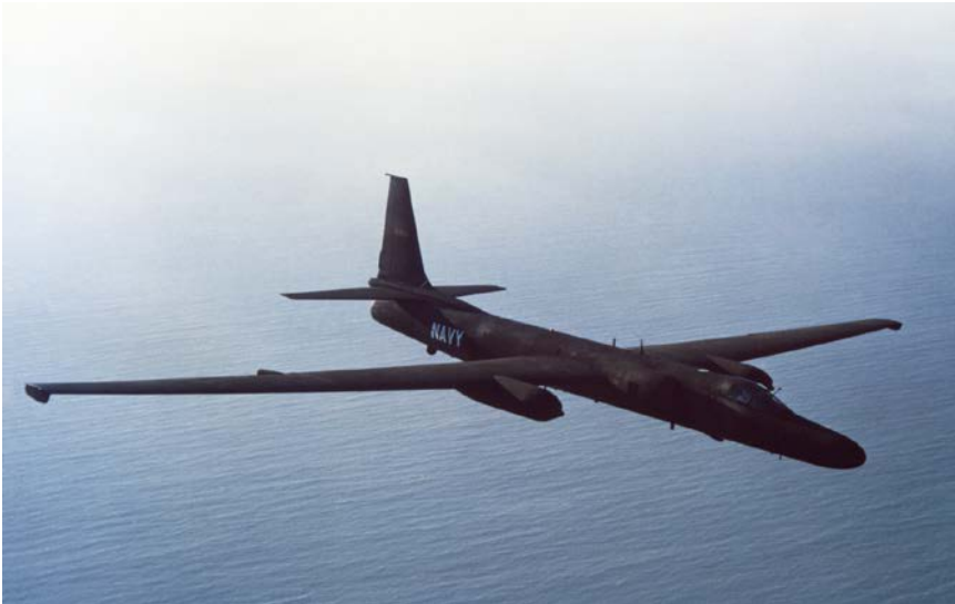
A U-2R was fitted with radar systems to detect oceangoing vessels for the Navy EP-X test program. (Lockheed Martin)
