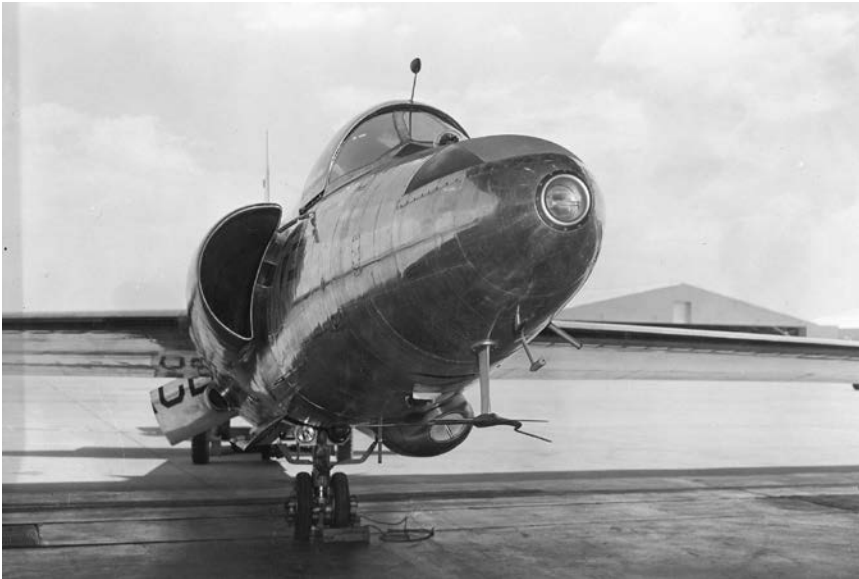
For the HASP mission, the U-2 was configured with a particulate sample in the nose and other instruments. (U.S. Air Force)
