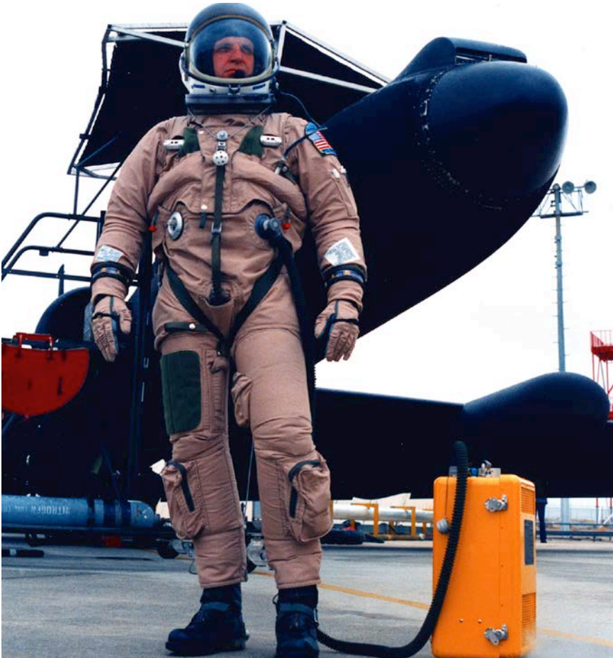
Lt. Col. Dee Porter demonstrates a prototype S1034 full-pressure suit at Palmdale in 1991. (Lockheed Martin)
