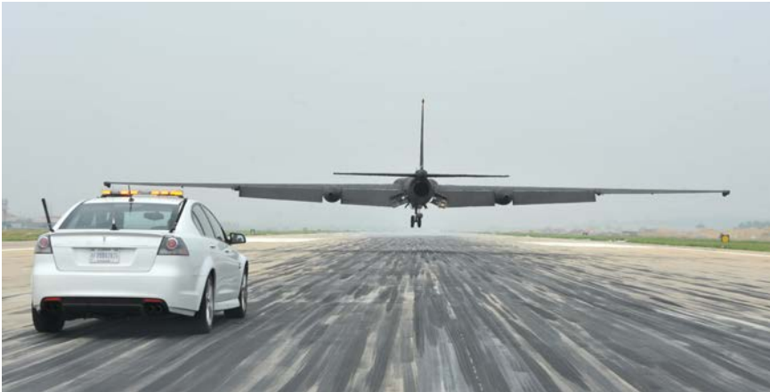
A mobile chase car follows a U-2 down the runway during landing. (U.S. Air Force)
