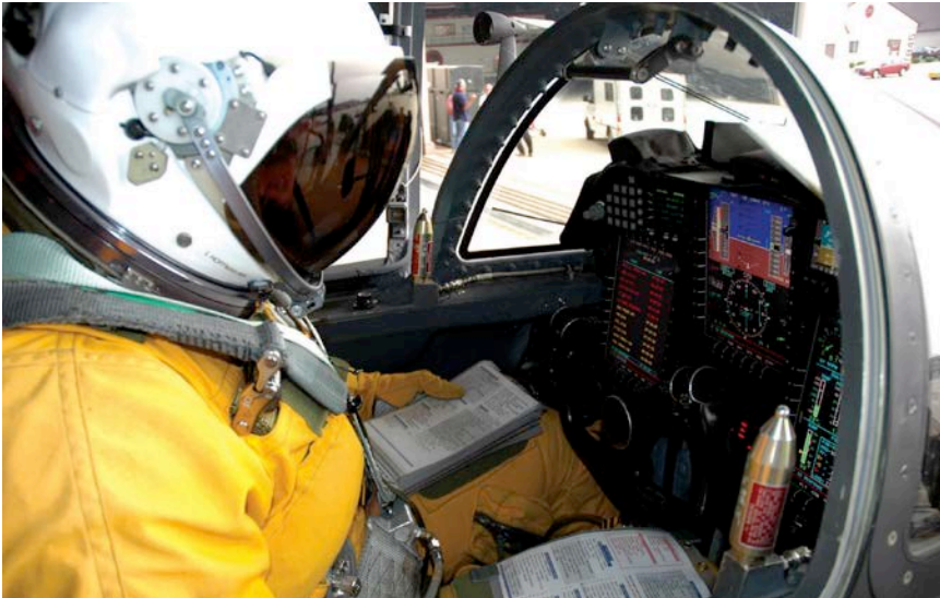
To reduce the chance of decompression sickness, cockpit upgrades have improved cabin-pressure altitude. (U.S. Air Force)
