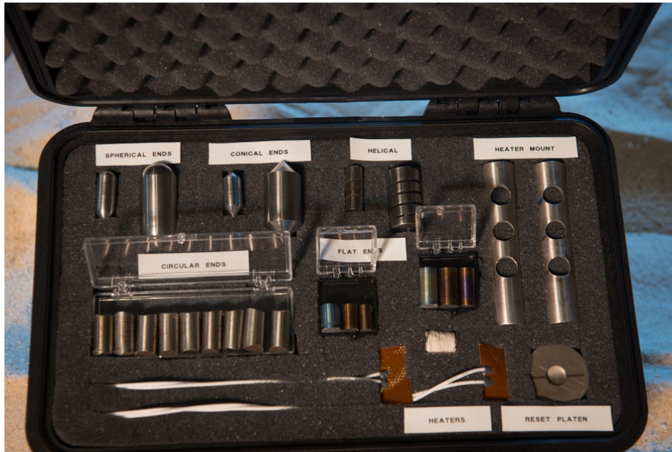
Figure 17.—SMARS prototype testbed and enclosure with temperature controller. (b) Prototype kit of several SMAs with different end-conditions, heaters, and resetting platens.
