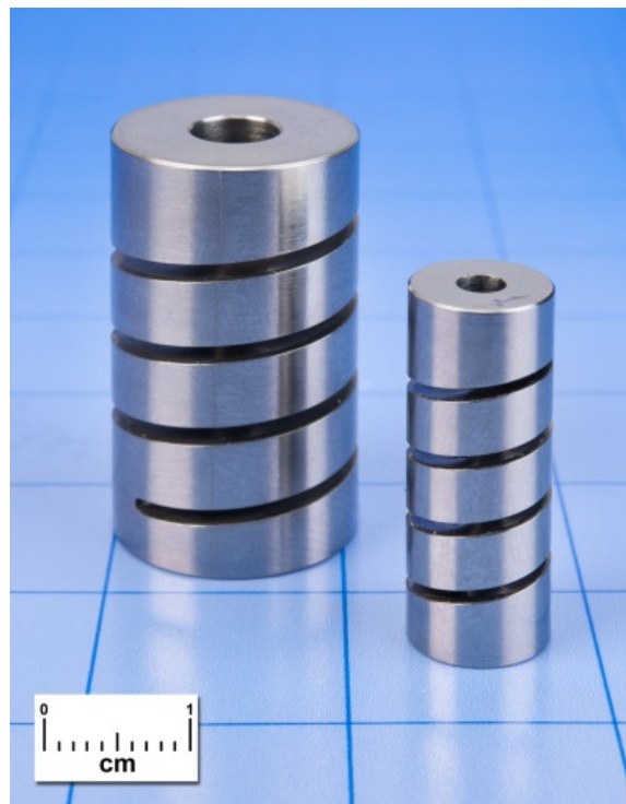
Figure 4.—Shape memory alloy helical pushers. End-tips can also be attached to this component.
