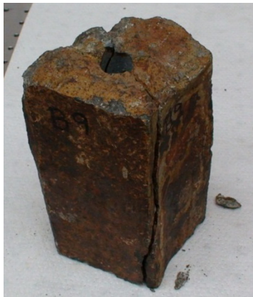
Figure 18.—Basalt test with \text{Ni}_{50.3}\text{Ti}_{29.7}\text{Hf}_{20} trained using the isobaric method under -200 MPa. The sample was placed \sim 2.5 in. deep within the borehole.
