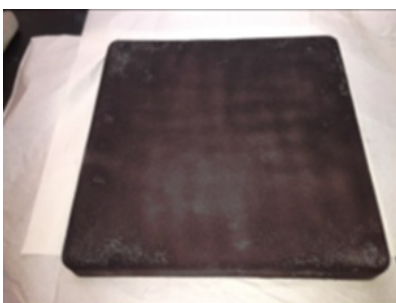
A high temperature resistant material was created using foamed basalt This paver was made of sintered basalt
