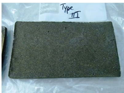
A high temperature resistant material was created using foamed basalt This paver was made of sintered basalt
