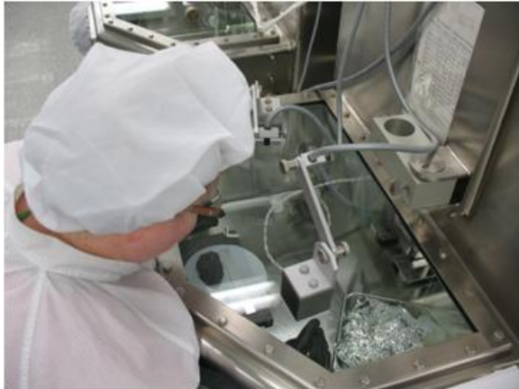
Figure 50: Lunar material being processed inside LCG during testing.
