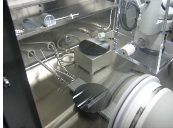
Figure 16: 2008 Balazs organic wafer testing on cold plate and weighing balance.
