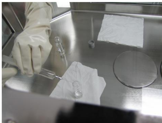
Figure 69: Collection of methylene chloride to the surface of the ACG with glass syringe.
