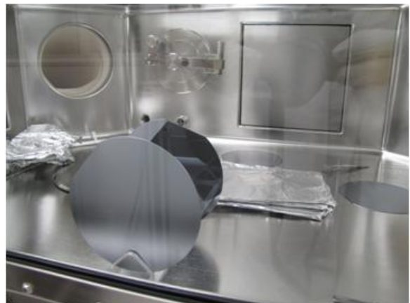
Figure 53: 6" silicon wafer vertical exposure in the ACG.
