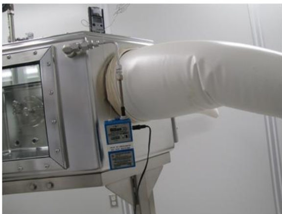
Figure 61: Location of adsorbent tube attachment to main chamber of the ACG.
