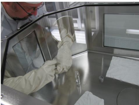
Figure 68: Application of methylene chloride to the surface of the ACG with glass syringe.
