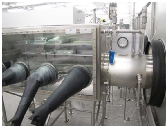
Figure 62: Location of adsorbent tube attachment to main chamber of the LCG.
