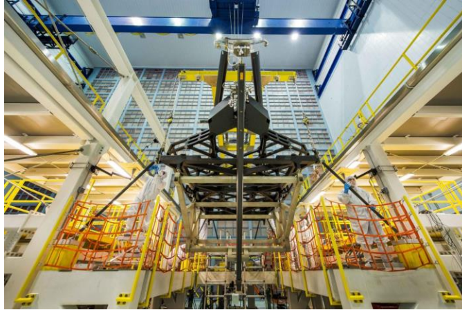
Figure 14: The Pathfinder is shown as it is being moved from the cart to the AOAS for mirror integration.
