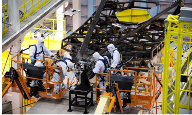
Figure 22: The secondary mirror was aligned using the SAIF while the integration team were suspended in JLG baskets for reach and access
