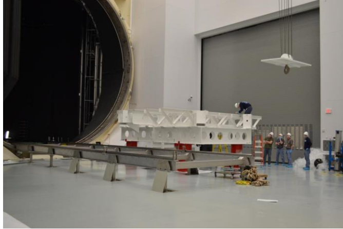
Figure 5: The JSC clean room will be used to stage the Pathfinder and flight system into the large refurbished cryo vacuum chamber.
