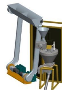
MARCO POLO • Soil dryer with regolith delivery and avionics • Water cleanup and storage
