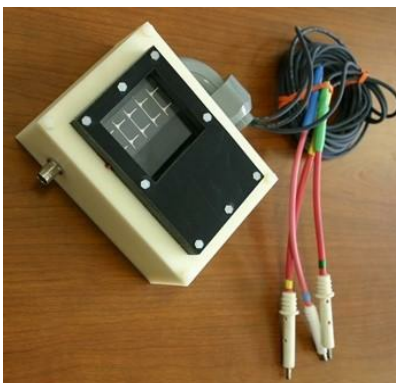
Early Prototype of EDS Lunar Experiment shown with Glass Shield and Solar Cells.
