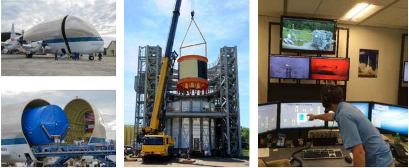
Figure 3: 5.5-m tank arrives on NASA's Super Guppy and begins testing at MSFC.
