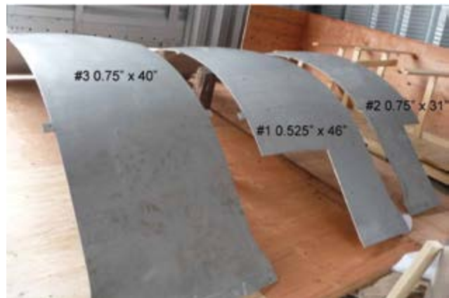
Figure 4: The three completed gore panels after delivery to MSFC. Test specimens were cut from the ends of two of the gore panels for mechanical and fracture toughness testing.
