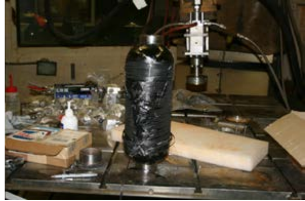
Burst testing (a) before burst and (b) after burst (failure in hoop).
