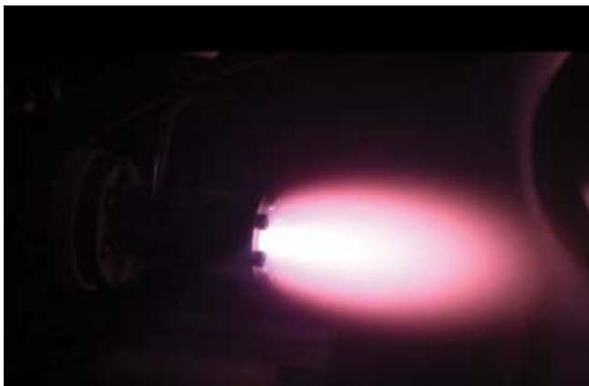
Figure 2: The direct drive arcjet in operation.
