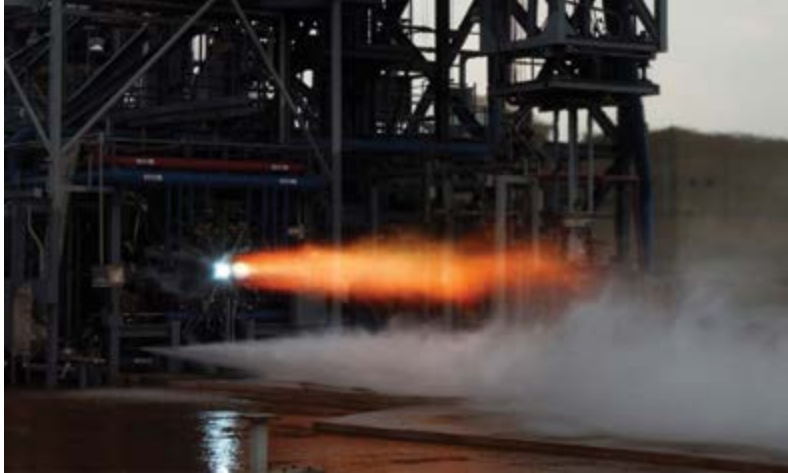
Example of a previous engine component testing at MSFC's Test Stand 116. Our hardware will be tested at similar liquid hydrogen and liquid oxygen flow rates and thrust levels.
