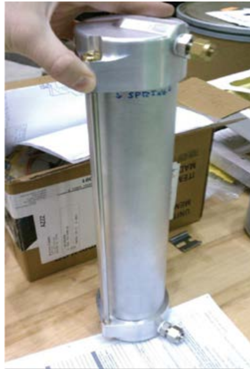
HMC source contaminant control sorbent bed.
