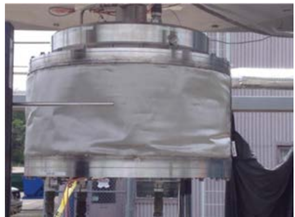
Low-profile diffuser being tested with wire-cloth attached using hot-wire anemometer to measure external velocity profiles.
