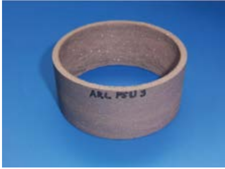
Figure 3: NARloy-Z-40vol% diamond composite cylinder fabricated by FAST.
