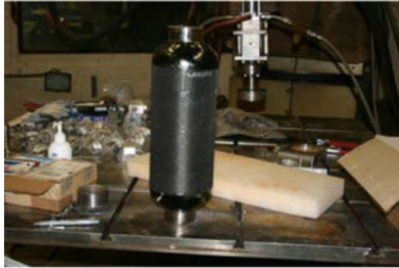
Burst testing (a) before burst and (b) after burst (failure in hoop).
