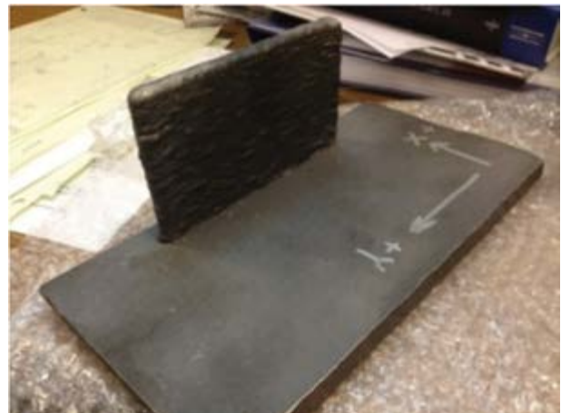
Figure 2: Preliminary build of Inconel 718 for mechanical property testing.
