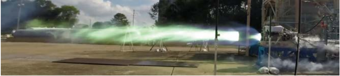
SWORDS engine testing at 75% power level.
