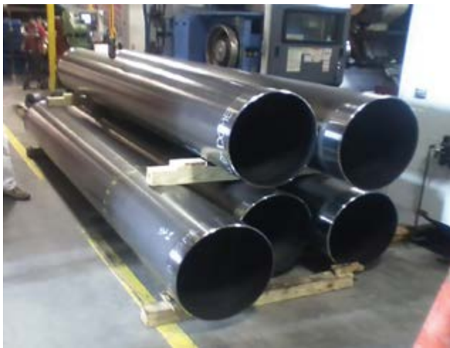
Motor cases ready for processing.
