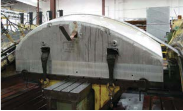
Figure 3: An aluminum panel is stretch formed into the desired contour using a die.
