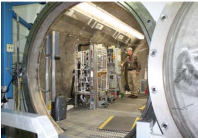
Integrated test chamber enables testing of AR technologies in an environment that simulates human metabolic activity integrated with functional AR hardware.
