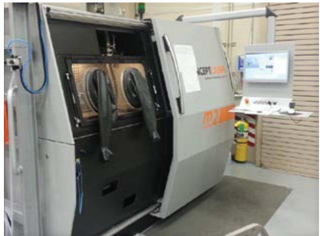
Figure 1: SLM machine with glovebox required for Ti64.
