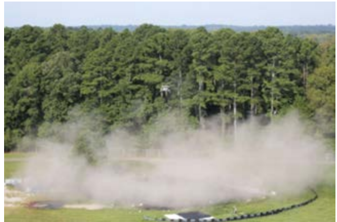
Dust being blown by a lander's rocket exhaust at the MSFC Lunar Terrain Testbed.
