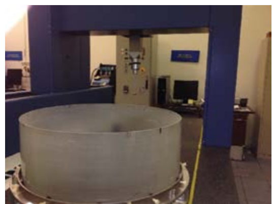
Figure 2: Thick glass shell on coordinate measuring machine.
