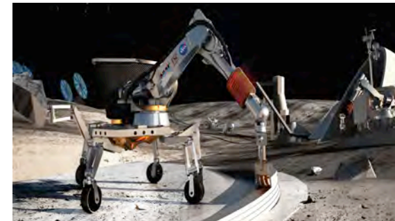
Concept of ATHLETE-based autonomous additive construction system on extraterrestrial surface. Courtesy: B. Khoshnevis, CCI
