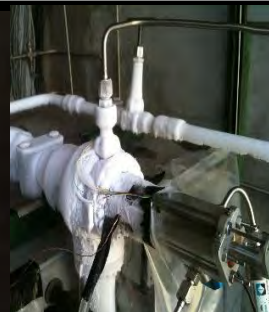
Main Fuel Valve Cryo Test
