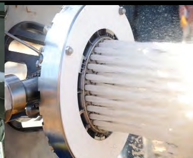
Full Scale Injector Water Flow
