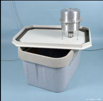
Photos of vault housing the sensor, digitizer and RF modem.
