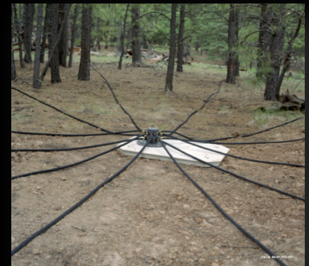
Deployed vault and sensor showing noise reduction hoses. This and three other sites make up the array.
