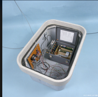
Photos of vault housing the sensor, digitizer and RF modem.
