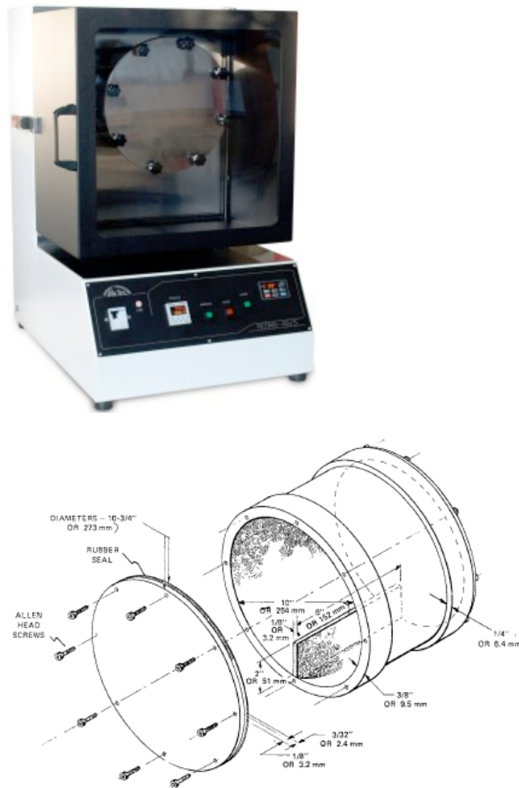
Figure 10. Attrition and Abrasion Test per ASTM Standard D4058
