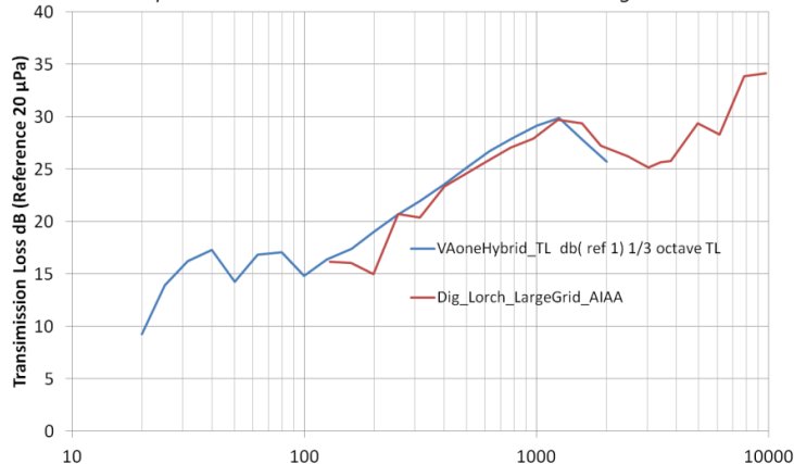
Isogrid Rib-Stiffened Panel Transmission Loss Estimate
