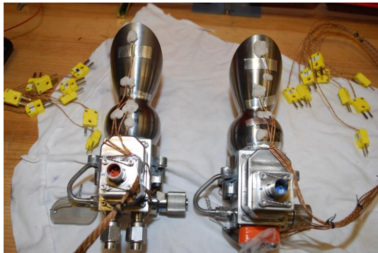
Figure 5: Instrumentation on the RS-34 thrusters for hot-fire test
