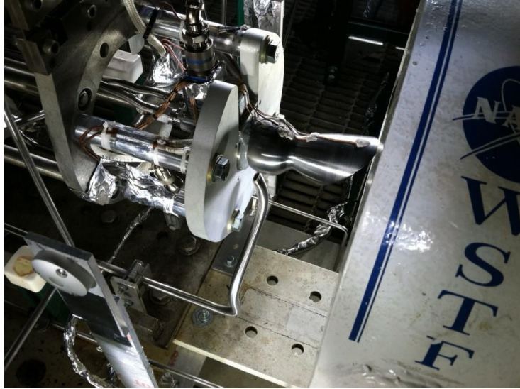
Figure 6: RS-34 thruster test setup in a vacuum chamber at WSTF
