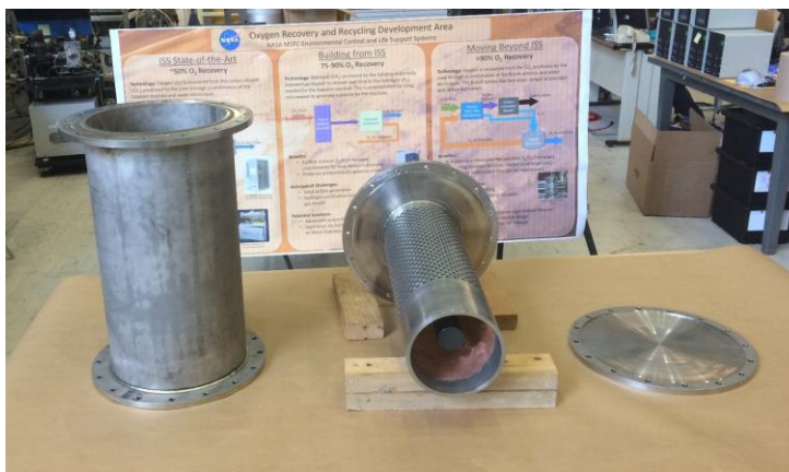
Figure 4. Fabricated Batch CFR. CFR shown in three parts: the outer (fourth) cylinder (on left), the reactor top cap connected to the perforated third cylinder covered with copper mesh and containing the second cylinder end cap (center), and the reactor bottom cap (right).
