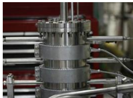
Figure 2. Reverse Water-Gas Shift Reactor with band heaters and integrated thermocouples.
