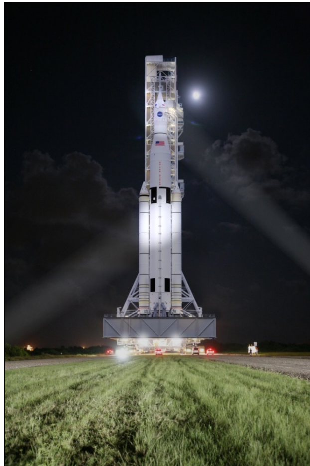
Fig. 1. Artist's concept of SLS aboard the Mobile Launcher moving to the launch pad.
