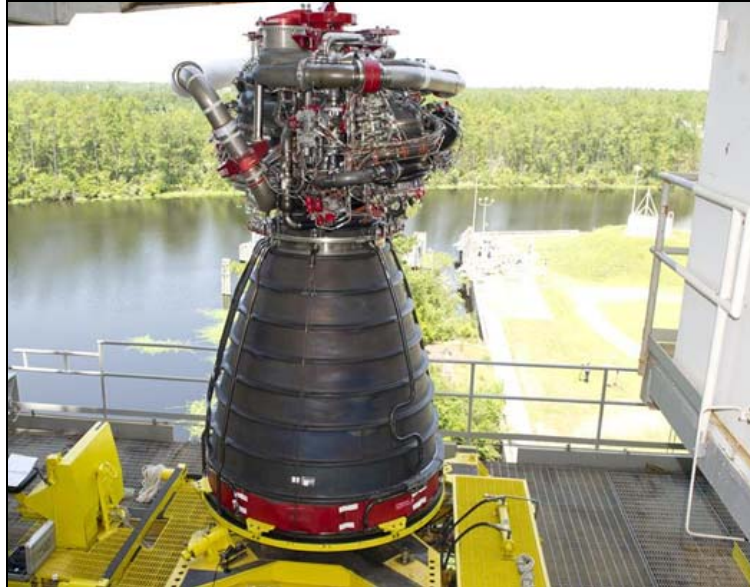
Fig. 5: RS-25 engine #0525 ready for installation on the A-1 test stand.
