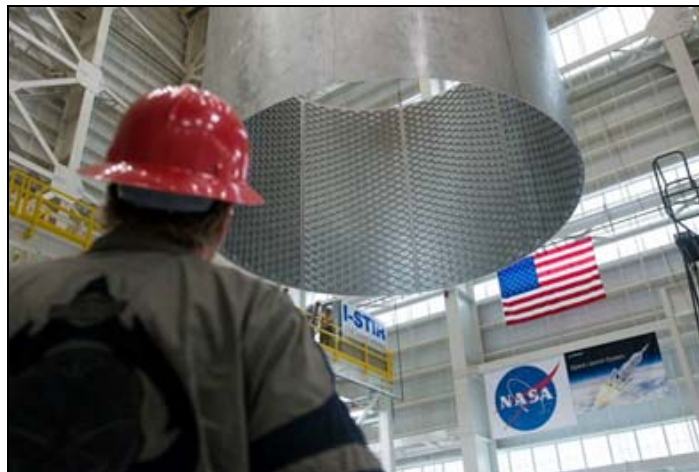
Fig. 4: Core Stage barrel section.
