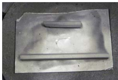
Figure 6: Graphite composite fuel element extrusion at ORNL
