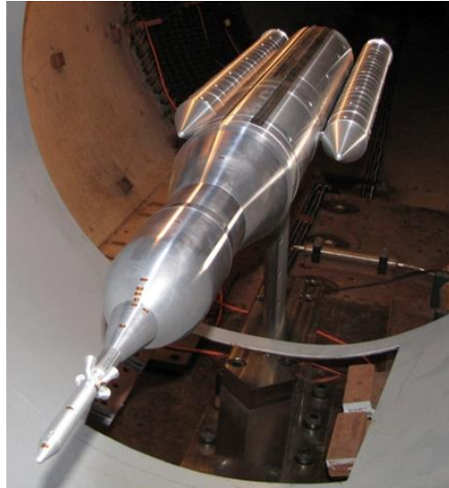
Figure 1. 2% scale hot-fire SLS model mounted in the LENS II tunnel
