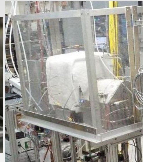
RWGS Reactor (following insulation and containment)
