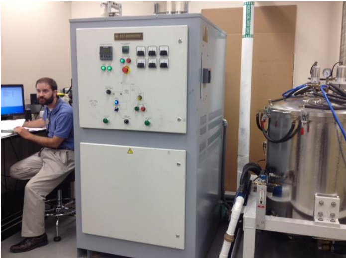
MSFC High Temperature Furnace
