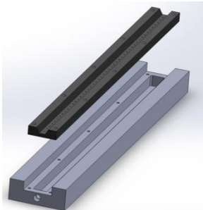
Right: Layoff base / Graphite insert
