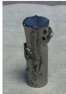
Above/left: Pure W sample post shakeout run 2. Sample reached melting point (3695K) and was held in place by the BN insulator.
