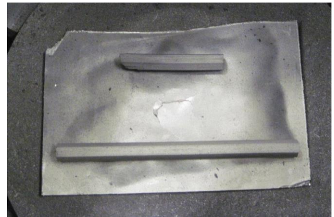
Initial ORNL graphite composite samples after the final heat treatment to 2700 C. Long sample is a section from an extrusion run. Short one is run out material left over from extrusion run. (Heat treated to have some extra material)
