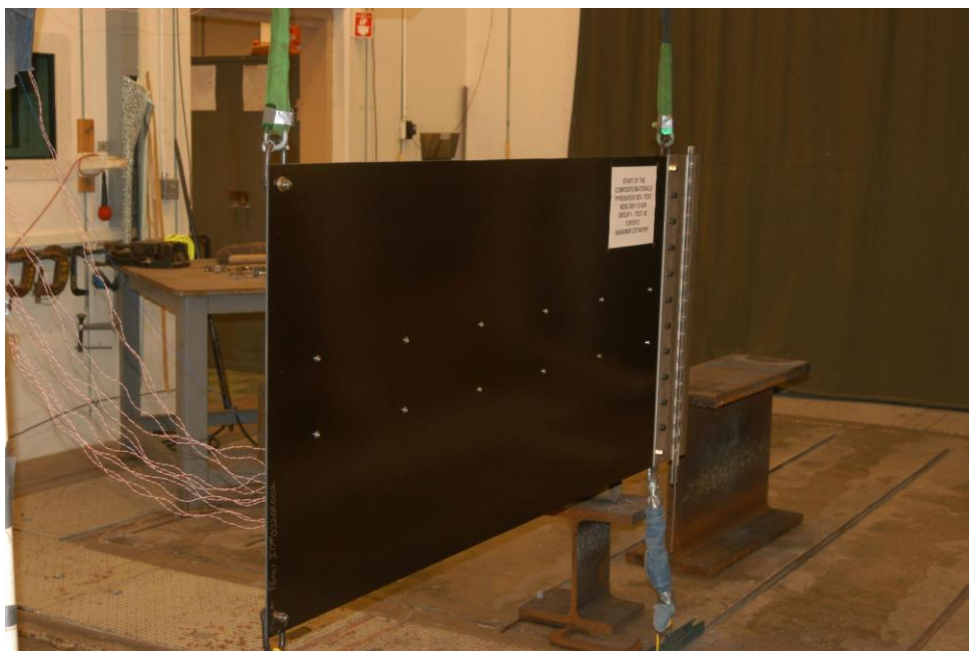
Figure 7.2.4.1-3. Monolithic Composite Panel Pyroshock Test Setup (Typical)
