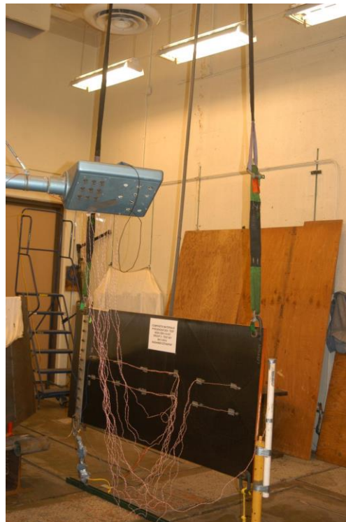
Figure 7.2.4.1-5. Composite Sandwich Panel Pyroshock Test Setup with Composite LSC Panel (Typical)
