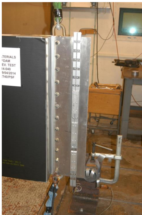
Figure 7.2.4.1-6. Composite Panel with Melamine Foam Pyroshock Test Setup (Typical)
