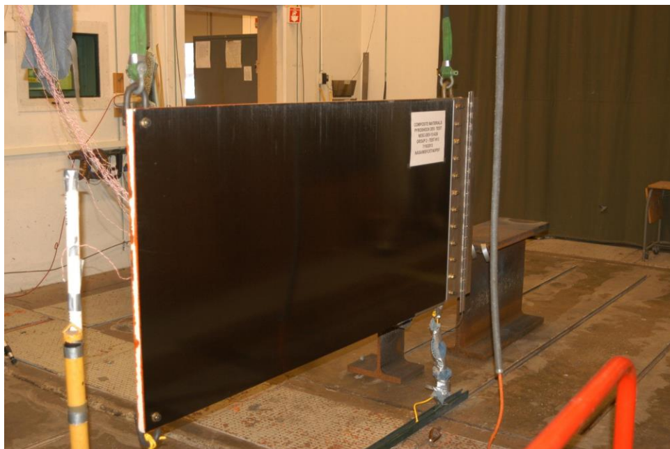
Figure 7.2.4.1-4. Composite Sandwich Panel Pyroshock Test Setup (Typical)
