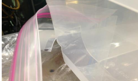
Figure 13: Image of the collection tub corner flap used to sweep FOD into Ziploc bag
