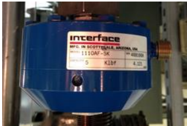
Figure 1: Image of the 5000 lb load cell
