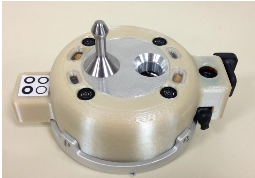
Figure 9: SDP has thin 3-D printed parts with fragile geometries shown in tan *
