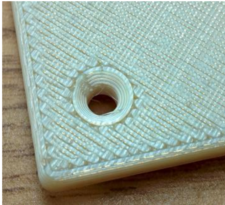
Figure 2: Images of the countersunk screw hole *
