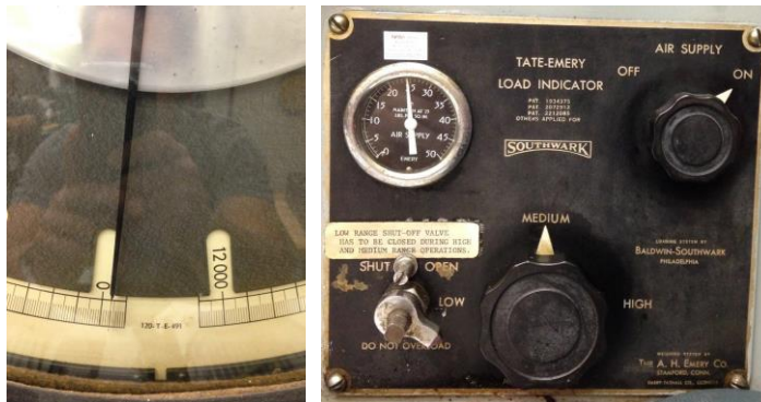
Figure 2 & 3: (Left) Force indicator set to 12,000lb max load. (Right) Image of the pressure gauge knob set to “medium”.
