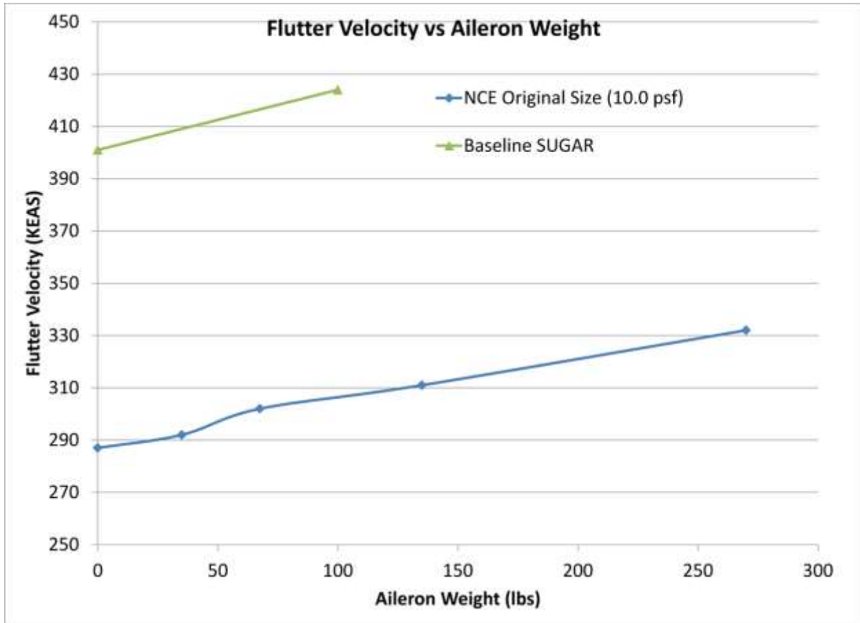
Figure 134. The effect on flutter velocity by adding weight to the aft portion of the wing. Results are shown for the baseline SUGAR wing, the baseline NCE wing, and a minimum gauge structure NCE wing. The trend seen is that flutter speed increases with the addition of aft weights. This result is contrary to typical behavior seen in a traditional cantilever wing (i.e., not a TBW).
