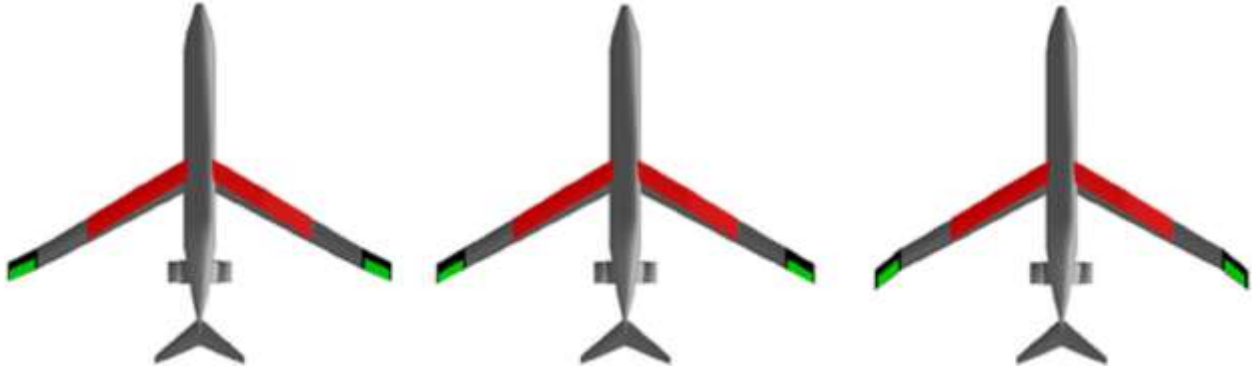
Figure 29. TBW Design1. From Left: (a) NCE Forward 5 deg (TBWdes1sf5), (b) NCE Unswept (TBWdes1as-is), (c) NCE Back 10 deg (TBWdes1sb10)
