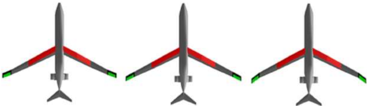
Figure 30. TBW Design 2. From Left: (a) NCE Forward 5 deg (TBWdes2sf5), (b) NCE Unswept (TBWdes2as-is), (c) NCE Back 10 deg (TBWdes2sb10)
