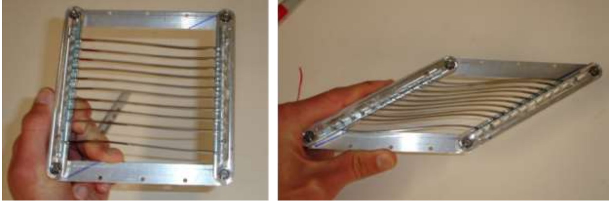
Figure 15. Shear cell used in previous NextGen morphing program with silicone skin removed to show flexible support blades.
