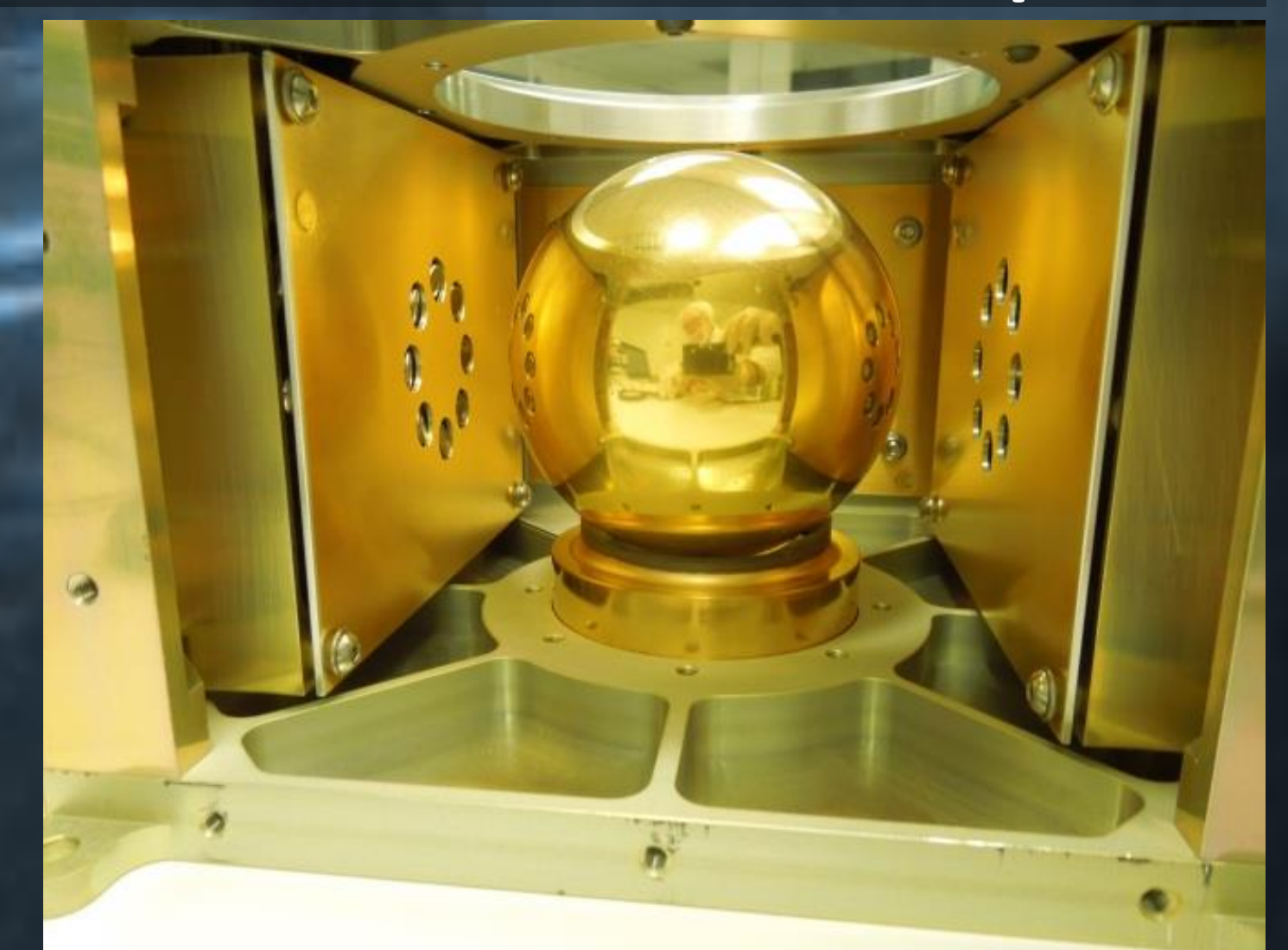
Figure 4. Interior of UV-LED, showing gold-coated proof mass and 2UV-LED boxes on either side
