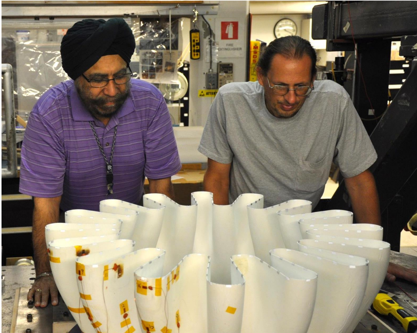
Visual Inspection of the Full Scale ERA Ox/Ox CMC Mixer 2014
