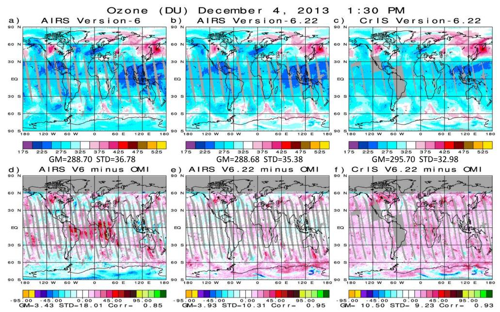
AIRS Version-6, AIRS Version-6.22, and CrIS Version-6.22 QC'd fields of total  $O_3$  for ascending orbits on December 4, 2013, and their differences from OMI. CrIS is missing parts of some orbits. AIRS V6.22 agrees much better with OMI than AIRS V6 with regard to both STD and spatial correlation. CrIS V6.22 statistics are comparable to AIRS V6.22 but CrIS is biased high.
