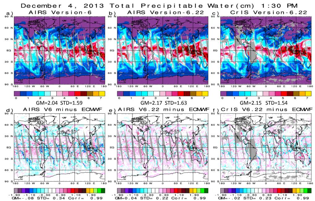
Derived QC'd fields of Total Precipitable Water ( $W_{TOT}$ ) for the ascending (1:30 PM) orbits of AIRS and CrIS, and their differences from the ECMWF 3-hour forecast for this time period, which we take as truth. AIRS V6.22  $W_{tot}$  is much more accurate than V6, especially in areas of high cloud cover. CrIS  $W_{tot}$  is very good as well.
