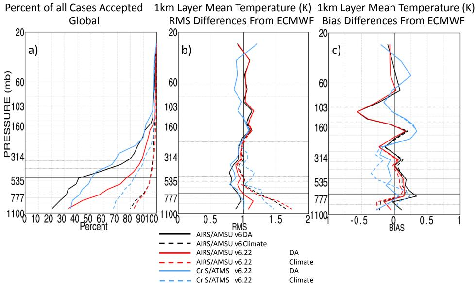
Global QC'd 1 km layer mean temperature profile statistics for December 4, 2013 for different retrievals and different QC thresholds. CrIS results use both the AIRS Version 6.22 DA and Climate thresholds. CrIS results using DA QC has a lower yield than AIRS Version 6.22 with smaller errors, as expected. CrIS results with Climate QC has a lower yield and larger errors than AIRS, possibly indicative of poorer performance in cloudier scenes than AIRS.
