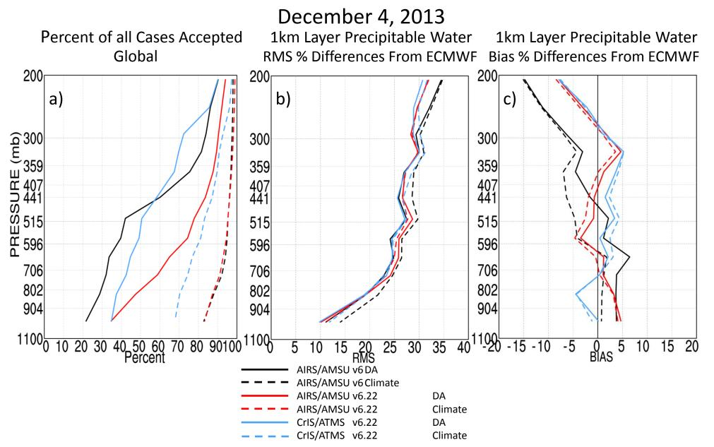
Global QC'd 1 km layer precipitable water profile statistics for December 4, 2013 for different retrievals and different QC thresholds. AIRS and CrIS Version 6.22 results are both superior to those of AIRS Version 6 with regard to both RMS errors and biases, especially with Climate QC.
