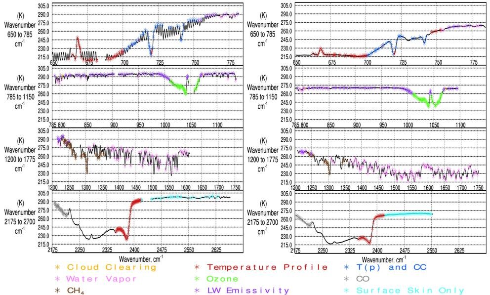
Sample AIRS and CrIS brightness temperature computed for cloud free scenes. The AIRS and CrIS channels we use in different steps in the retrieval process are indicated in the figures by different colored stars. AIRS is sampled twice as densely as CrIS.
