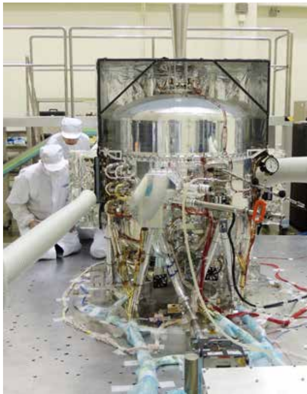
The finished SXS dewar undergoing vibration testing at the Tsukuba Space Center in Japan.
