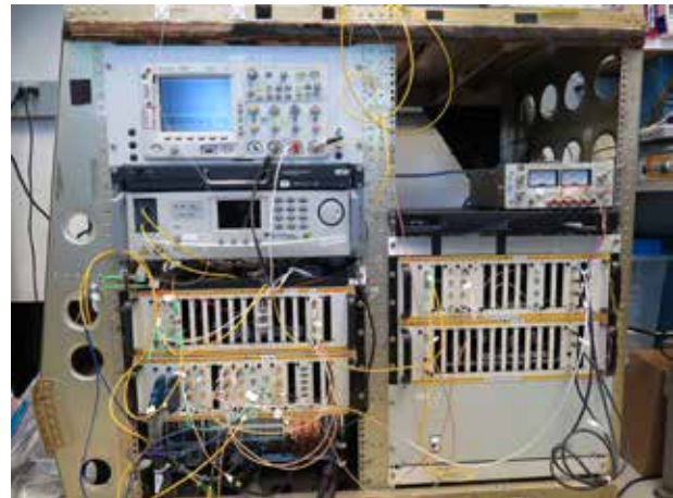
Seed laser rack for ASCENDS flight campaign
