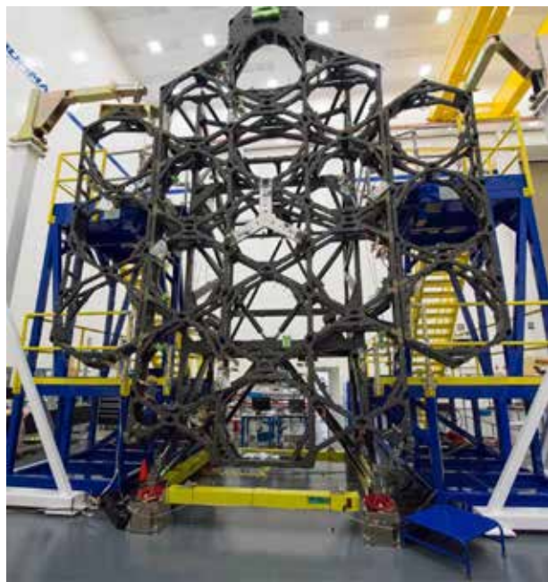
The JWST flight backplane center section and side wings were assembled in 2014 and will be delivered to Goddard in 2015. Credit: Northrop Grumman
