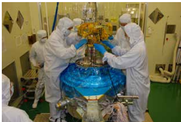
Scott Porter and Meng Chiao (front left and right) assist with the installation of the flight SXS Calorimeter Spectrometer Insert into the flight dewar.
