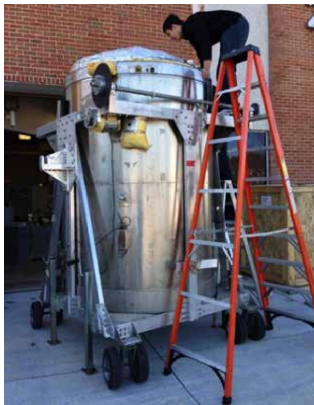
The PIPER flight dewar is a 3-meter-tall “flying cold tub” containing 3500 liters of liquid helium.
