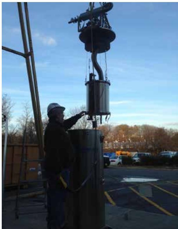
The PIPER detector electronics are lowered into a cryostat for testing.
