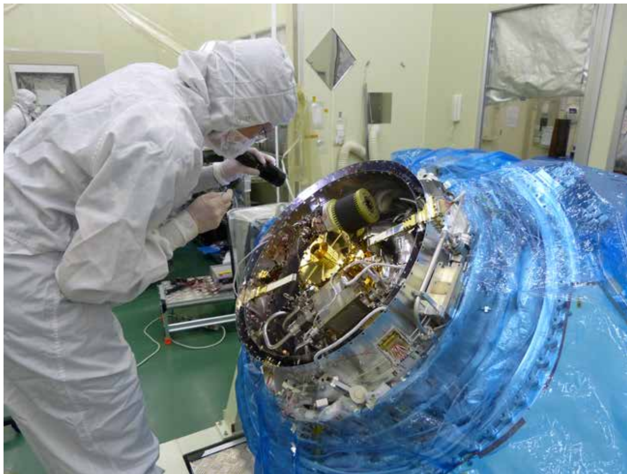
Caroline Kilbourne inspects the completed forward end of the SXS dewar prior to the next phase of close out and aperture installation.
