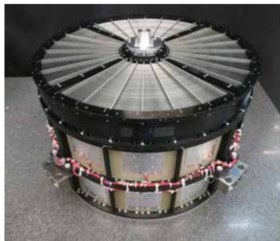
The X-ray mirrors produced for the Astro-H Soft X-Ray Imager (left) and SXS (right). The mirrors have 203 concentric reflectors, so contain 1624 individual, precisely aligned mirror segments. They are 45 cm in diameter and have a mass of 43 kg each.
