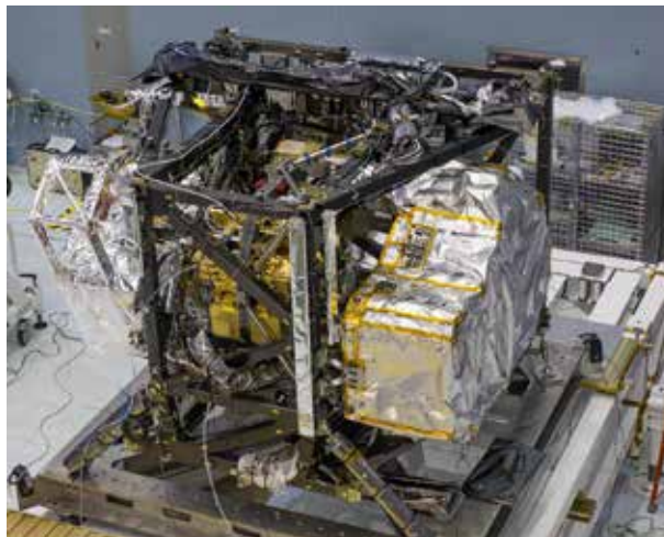
The JWST flight Integrated Science Instrument Module was fully assembled with all four instruments and underwent a cryogenic vacuum test in 2014. Credit: NASA/Chris Gunn
