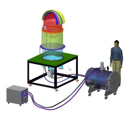
Launch Pad Ground Support Cryocooler
