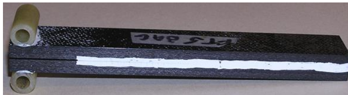
Figure 1. DCB test specimen with 2.5-inch flaw.
