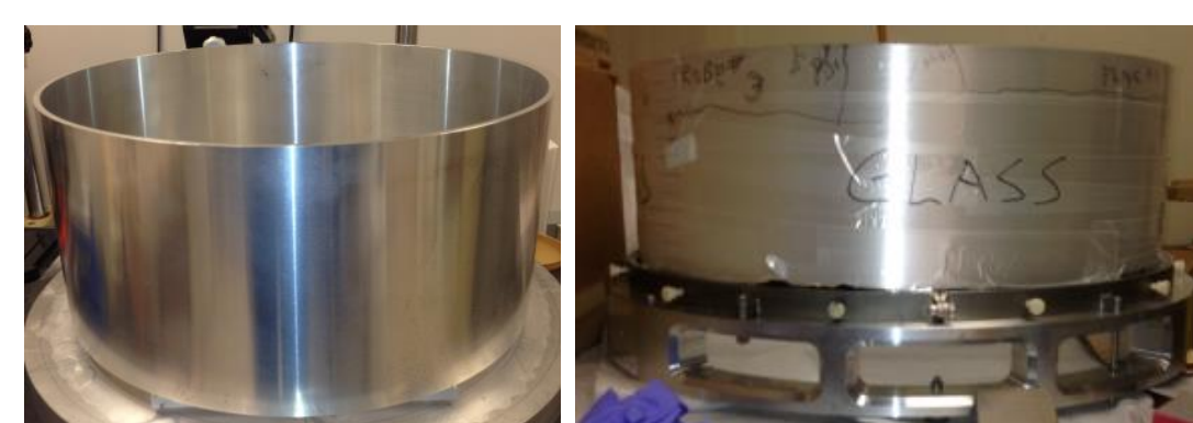
Figure 2. Aluminum (left) and glass (right) substrates for the direct fabrication of high resolution x-ray optics
