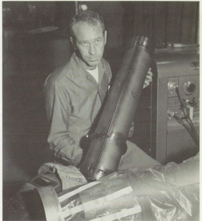
Fig. 4. Completed Weldment of Titanium-Alloy Motor Case
