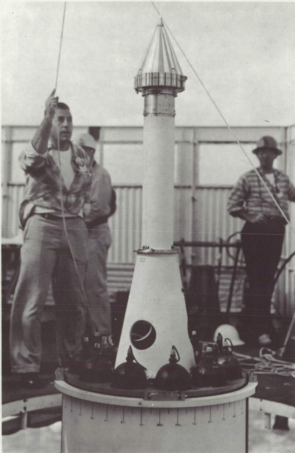
Fig. 1. Moon-Probe Vehicle, Showing Pioneer IV Mounted on Titanium-Cased Fourth-Stage Rocket Motor
