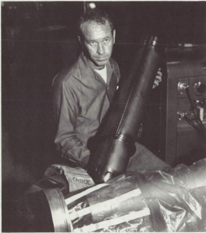
Fig. 4. Completed Weldment of Titanium-Alloy Motor Case
