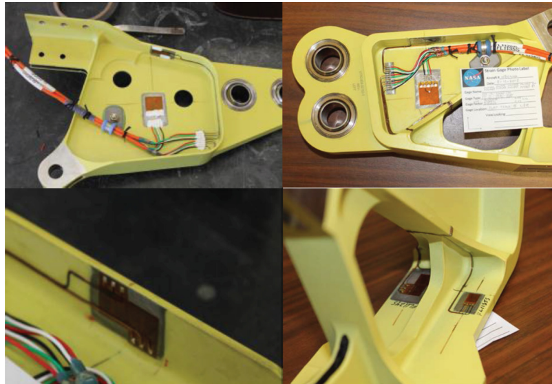
Figure 14. ACTE interface fitting strain gage installation.
