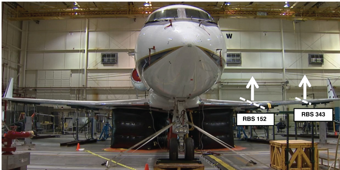
Figure 11. Photograph of hydraulic up load case with aircraft supported on airbags.
