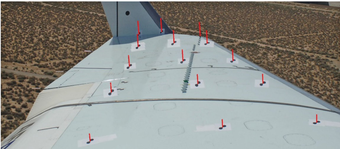
Figure 17. GIII wing deflection measurement system.
