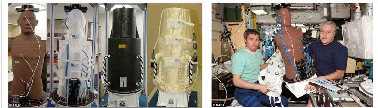
Figure 13. Mannequins serve as radiation test subjects collecting data without risk to astronauts.
