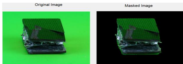
Fig. II: This section of composite panel was used as a test sample to assess the effectiveness of object detection for the types of fragments expected from DebrisSat. The object has a significant amount of green reflection and yet is still effectively detected by the algorithm.
