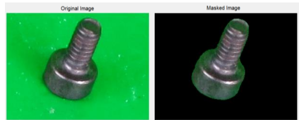
Fig. III: Fragments as small as this M2 socket head cap screw can be detected. This meets the research objective of characterizing fragments with characteristic lengths as small as 2 mm.
