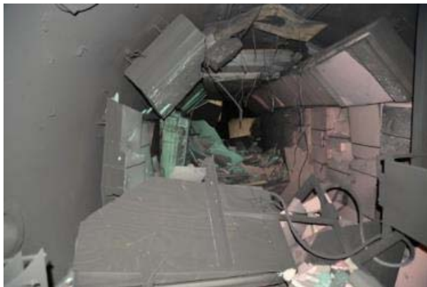
Fig. 4: Test chamber post-impact
