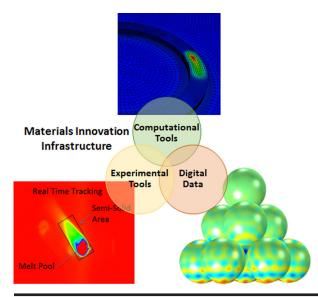
Physics-based models of powder consolidation, in-situ monitoring of the melt process and 3D models of the thermal history are used to predict material evolution and material behavior.
