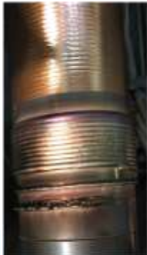
3.5" OD copper tube with In625 deposited on the surface
