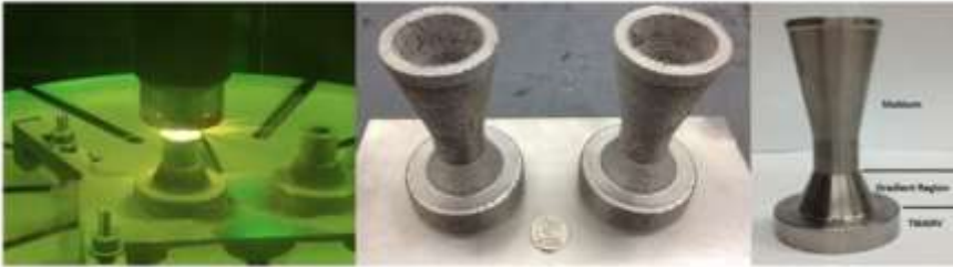
Prototype titanium to niobium gradient rocket nozzle
