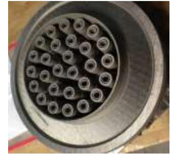
28-element Inconel 625 fuel injector
