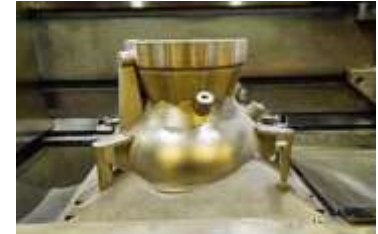
28-element Inconel 625 fuel injector
