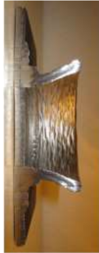
Cutaway of a 1.5" tall x 2-3.5" diameter (tapered) 316SS
