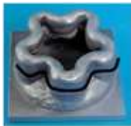
2219 Al mixer, 2.5" diameter, ~0.75" high (available parts are just the bottom half of this part, below line shown in photo)
