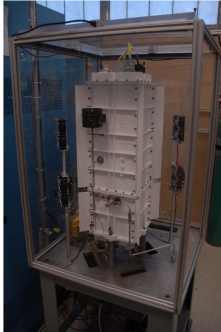
Figure 1. ASRG Engineering Unit Test Rig at GRC Stirling Lab.
