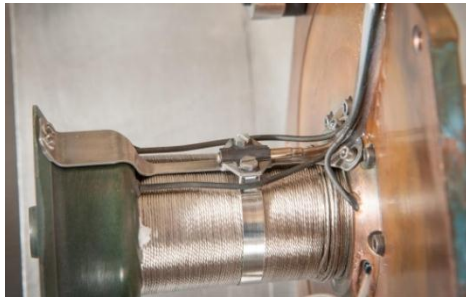
Figure 6. RTD Installation on the ASC.
